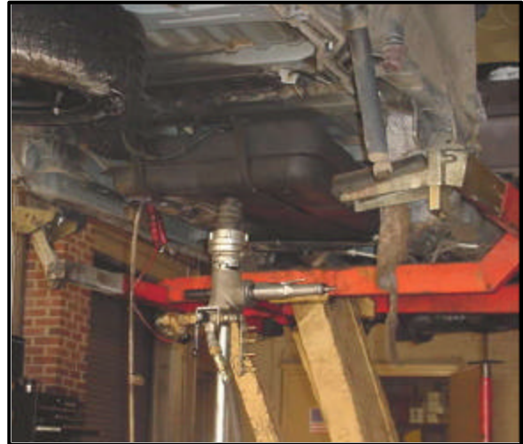
Removing gasoline with a tank drilling machine
