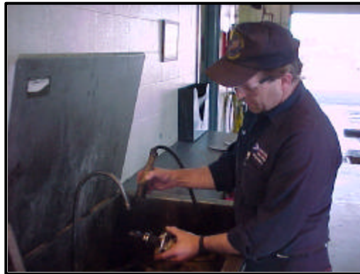
Using an aqueous-based parts washer
