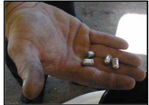
Mercury switches removed from vehicle light assemblies
