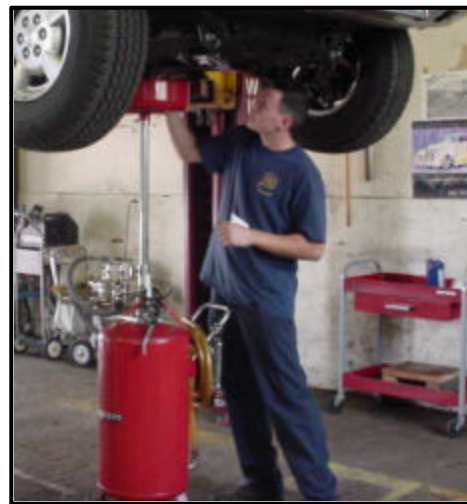
Vacuum-type drain system
