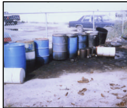
Improper used oil storage: leaking, unlabeled drums on ground
