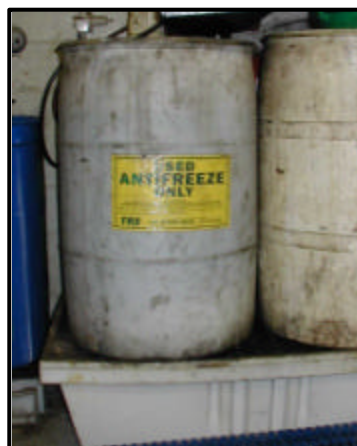
Used antifreeze, labeled and stored on secondary containment
