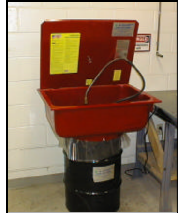
Solvent Parts Washer (lid should be closed when not in use)
