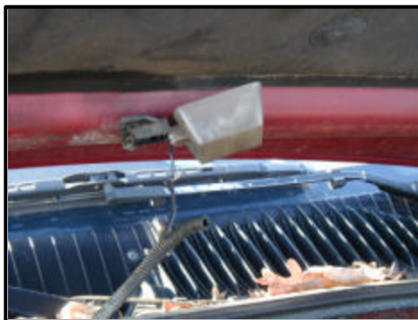
Hood light fixture with mercury switch assembly
